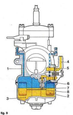
It is important that this level is always costant throughout the operating range because, with a costant depression in the venturi, a rise in the float chamber level would cause an increase in fuel delivery and consequently enrich the mixture; conversely, lowering of the float level causes a weakening of the mixture.
