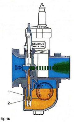
The channel size (4) is such that it creates an optimum vacuum in the starter valve chamber, at the emulsion tube otlet both for starting up and for the misture required by the engine for its running and warming up. Therefore, varying the position or the size of the starter emulsion tube holes will change the amount of fuel delivered; the mixture ratio is controlled by the starter jet size and therefore a larger jet causes enrichment and vice-versa.
