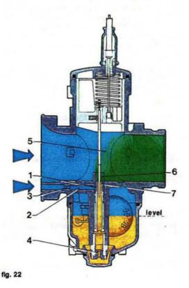
Usually the atomisers on carburettors intended for two-stroke engines are manufactured in two types: with either **long** or **short** upper parts (figure 23). The atomisers with **longer** upper parts cause a weakening of the mixture at low speeds and during acceleration from low speed; on the other hand, atomisers with **shorter** upper parts produce extra enrichment. Carburettors for racing motorcycles use atomisers with short upper parts.
